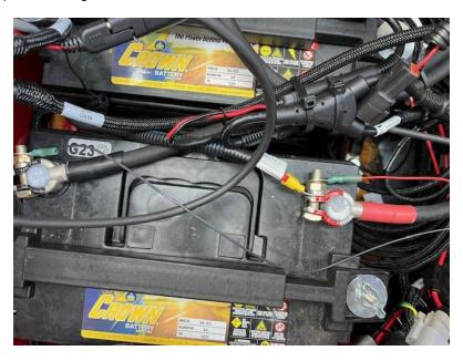
8. Verify the 10-amp fuse on the power side is present and seated properly.
