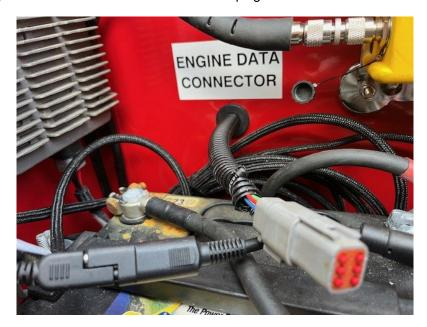
5. Connect the mating Deutsch connector on the RDO harness into the engine data harness.
