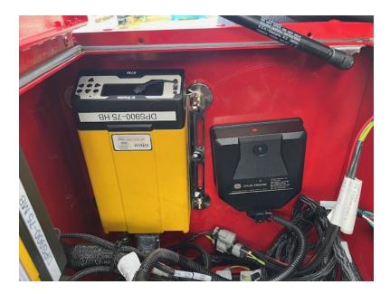
7. Connect the power portion of your RDO harness to the machine's batteries in a 12V configuration using the provided ring terminals. Terminals will need to be heated to seal the heat shrink.
