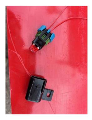
9. Connect the two-pin power connector from the battery harness to the RDO wiring harness.
