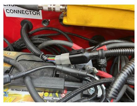
6. Plug the RDO wiring harness to M Modem and place the Modem next to the Trimble Controller using the 3M adhesive tape on the bottom of the Modem. \*Make sure the surface has been cleaned with glass cleaner or similar fluid to remove dirt/debris\*
