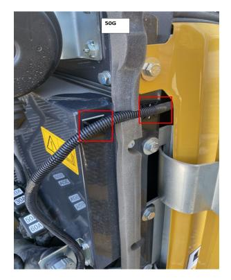
8. Make sure all wiring is tidy and secure away from hot points, pinch points and not obstructing radiator air movement. Use all zip tie adhesive plates. \*Be sure to use heat shrink wire nut ends if both plug-in ports are not available\*
