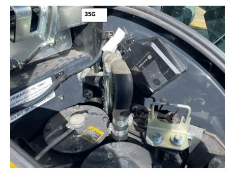
7. Route the cable starting in the hydraulic oil compartment-run the cable through the door hinge of the radiator/battery door. Pull all slack cable into the radiator compartment area. For the 50G-Use the Zip tie adhesive plates to secure the cable on each side of the foam. For the 35G's cut a slit into the thick foam and feed the cable through the foam in the same location as shown below.
