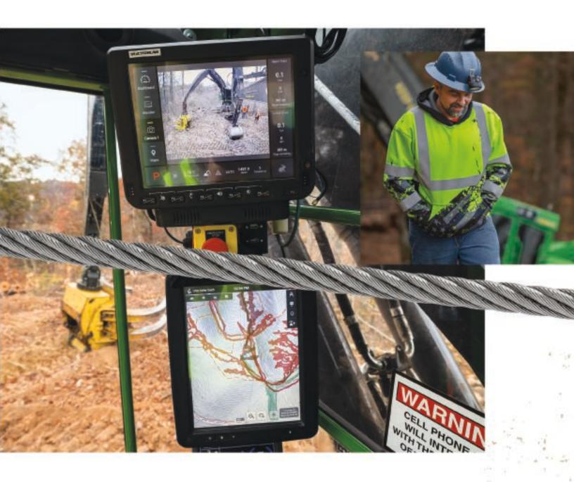
As the job progresses, the system also tracks tree-cut locations and inventory, and displays the locations and travel history of the shovel loader and skidder. The harvest plan can be updated immediately and continuously. "TimberManager and TimberMatic Maps make it so easy to update the information," says Moore. "Plans always change, and we can provide updates to the operator in the machine in a matter of minutes."
