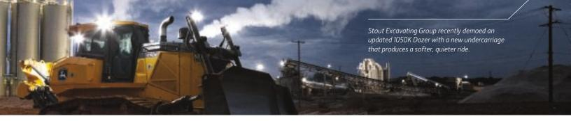
means of extraction from pits that can be over 100-feet deep. At pit number three, a John Deere 1050K Dozer maintains stockpiles, builds ramps, and shapes haul roads. A Deere 870G LC Excavator loads a continuous stream of Deere 410E ADTs, which haul the sand to a processing area where a Deere 944K Hybrid Loader feeds the hoppers.
